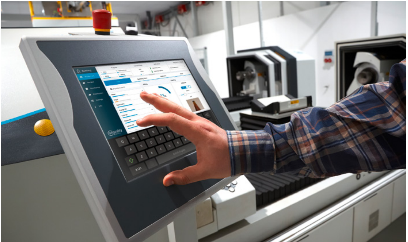
Figure 10: The HTML5 sequality- Bottling demo in QtWebView on an embedded Linux terminal.
